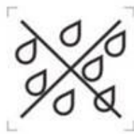
Figure 6 – Lamp not suitable for use under dust and moisture
